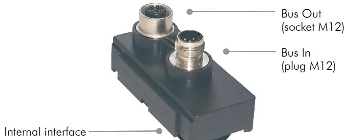
The RIO-P F CAN field bus module is plugged onto the RIO-P BC CAN DN or RIO-P BC CANopen bus coupler. It has an internal interface to the respective bus coupler and two M12 interfaces to the field bus. The M12 connectors correspond to IEC 947-5-2 with mechanical standard coding. The connections are in the module, so the field bus remains functional even if the module is removed.
