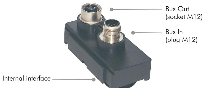
The RIO-P F DP field bus module is plugged onto the RIO-P BC DP bus coupler. It has an internal interface to the bus coupler and two M12 interfaces to the field bus. The M12 connectors correspond to IEC 947-5-2 with reverse key coding. The connections are in the module, so the field bus remains functional even if the module is removed.
