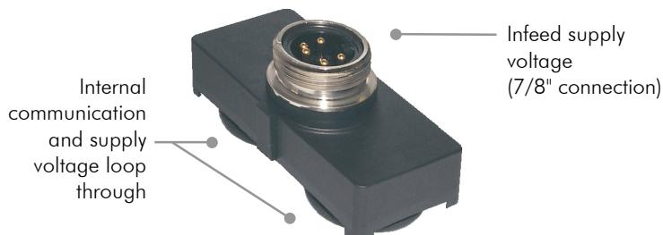
The infeed module feeds the supply voltage for the bus coupler module and the sensors and actuators via a 7/8" connection. It connects the bus coupler module to the first I/O module or connects two I/O modules.
